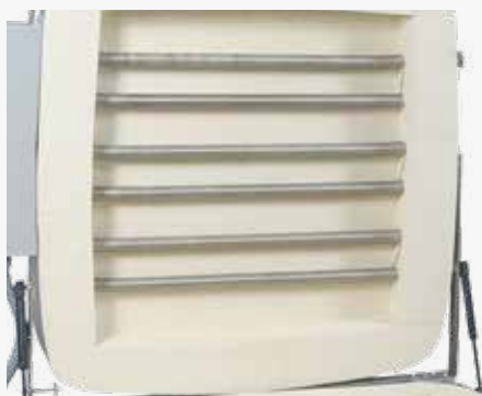
Heating on support bars
