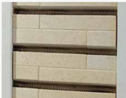
Heating elements in grooved bricks
